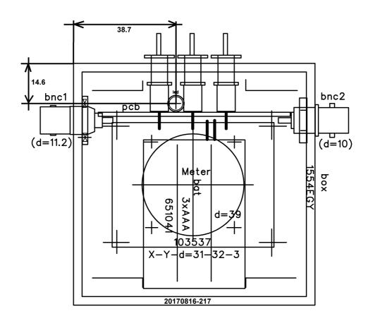
For easier installation of the PCB, the LED hole could be drilled into the top, and the switch holes as 6.2 mm,
