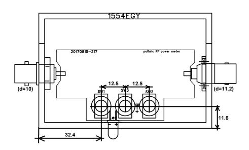
For easier installation of the PCB, the LED hole could be drilled into this top side, and the switch holes as 6.2 mm.
