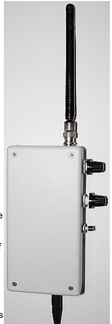
The above shown small ferrite rod (Conrad 535575) nicely fits inside a small 8.5cm x 17cm x 3cm Hammond 1599 ABS box. A 50x20x20mm piece of square ALU pipe could function as **sense antenna**, screwed on top of the box.
